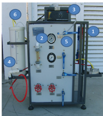
Fig. 2. Frontal view of the MF/UF module (Operation manual – MF/UF module): (1) polymeric membranes; (2) pressure gauges; (3) speed controller; (4) feed tank; (5) valve used to collect the permeate; (6) tubing through which the concentrate returned to the feed tank.
